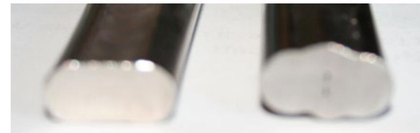
**TIG** where the two parts jointed are no more visible why a real melting is made and the two partstogether with the adding material generate a new component witout air boubles
